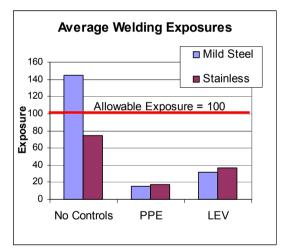
Contrary to what many welders believe, welding on mild steel results in higher exposure than welding on stainless steel. That is because up to 95% of the exposure is from the welding wire and not the metal being welded.
